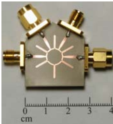
Fig. 4. Photograph of the dual-band rat-race.
