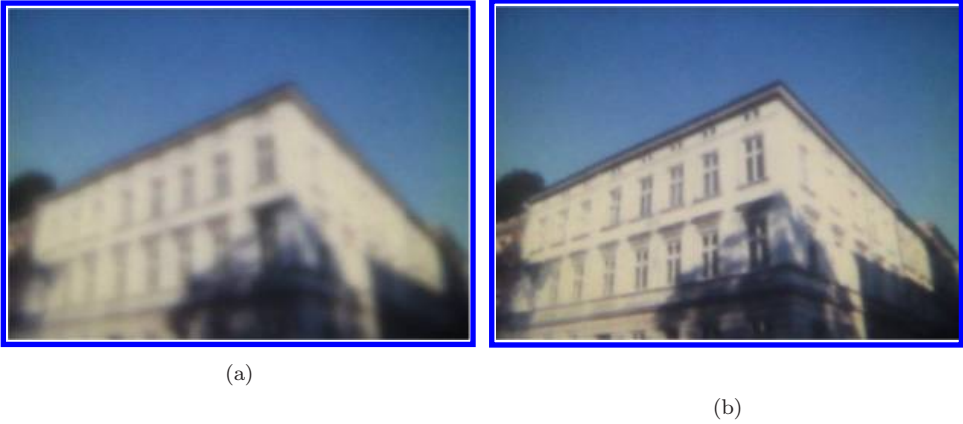
Fig. 4. The images of electrically tunable focusing LCOS pico projection system at (a) 0 V_{\text{rms}} and (b) 27 V_{\text{rms}} . The screen was placed 8 cm away from the LC lens.
