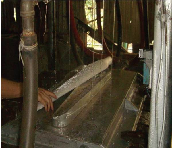
Fig. 2 Mold for fabricating PVC core
