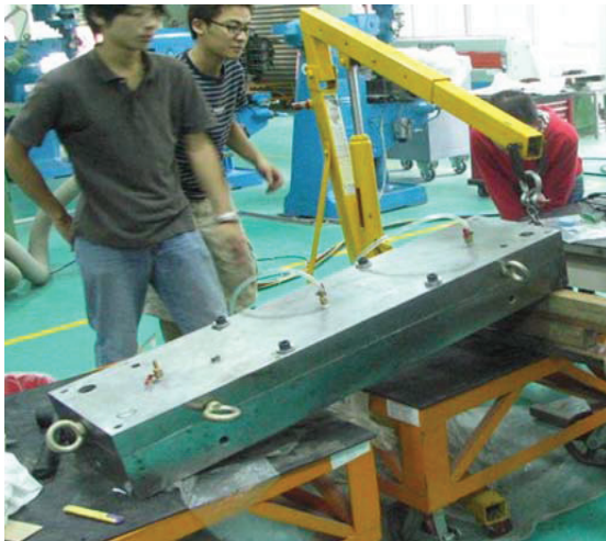
Fig.4 Steel mold for VRTM
