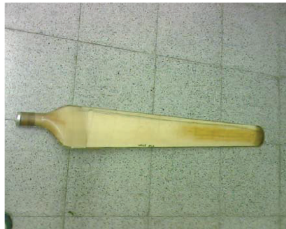
Fig. 5 Cured composite wind blade
