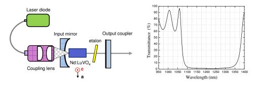
Fig. 3. Schematic of the experimental setup for the dual-wavelength Nd: $LuVO_4$  laser. Right: Measured transmittance curve for the output coupler.
