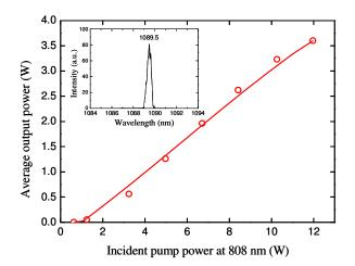
Fig. 4. Average output power versus the incident pump power for single-wavelength operation. Inset, optical spectrum of single-wavelength operation at the maximum output power.
