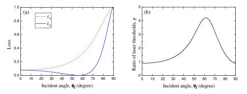
Fig. 2. Calculated results for the dependence of (a) the losses for S and P waves and (b) the ratio of laser thresholds on the incident angle for dual-wavelength operation.
