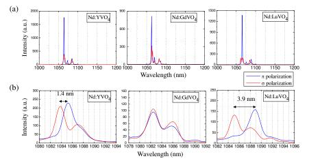
Fig. 1. (a) Fluorescence emission spectra for the  ${}^{4}F_{3/2} \rightarrow {}^{4}I_{11/2}$  laser transition in the Nd:YVO<sub>4</sub>, Nd:GdVO<sub>4</sub> and Nd:LuVO<sub>4</sub> crystals at room temperature; (b) fragments of the room-temperature fluorescence spectra near 1080 and 1090 nm.
