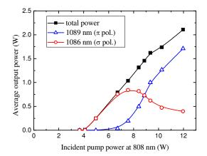
Fig. 5. Average output powers versus the incident pump power for dual-wavelength operation.
