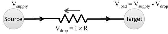
Fig. 2. IR-drop: considering a simple power supply system with a source supply current with the voltage V_{supply} , the target receives the voltage with only V_{load} = V_{supply} - V_{drop} .
