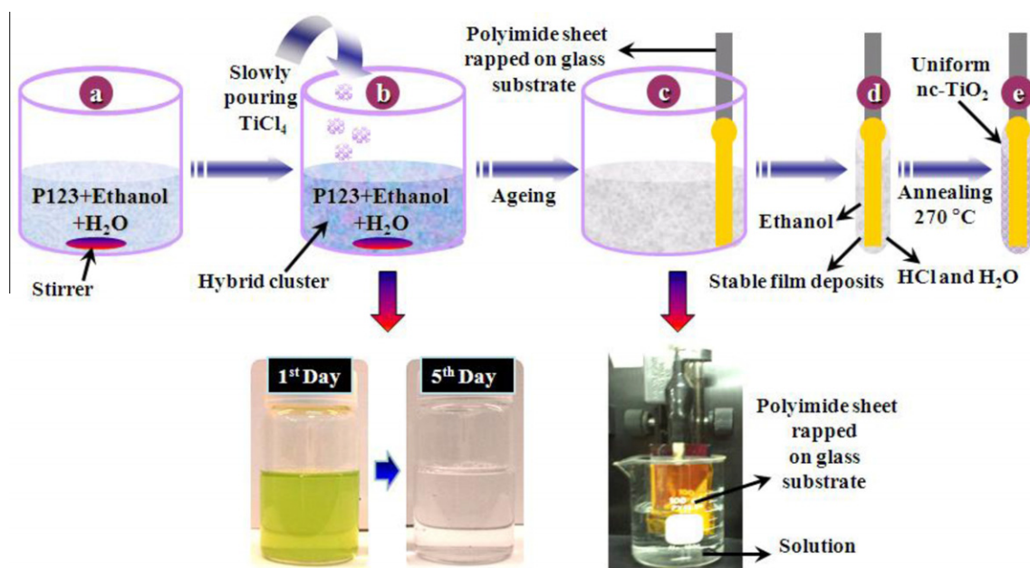
Scheme 1. (a–e) Schematic illustration of the proposed synthetic solution and dip-coating approach for the uniform preparation of the nc-TiO 2 film throughout this work.
