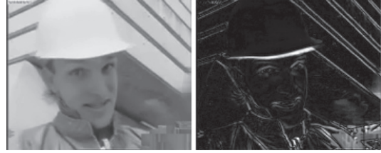
Fig. 12. The SI frame of the proposed codec (left) used in Fig. 11, and its error image (right). The SI frame of the DISCOVER codec is not available.
