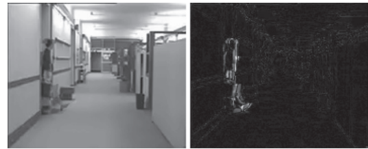
Fig. 16. The SI frame of the proposed codec (left) used in Fig. 15, and its error image (right). The SI frame of the DISCOVER codec is not available.
