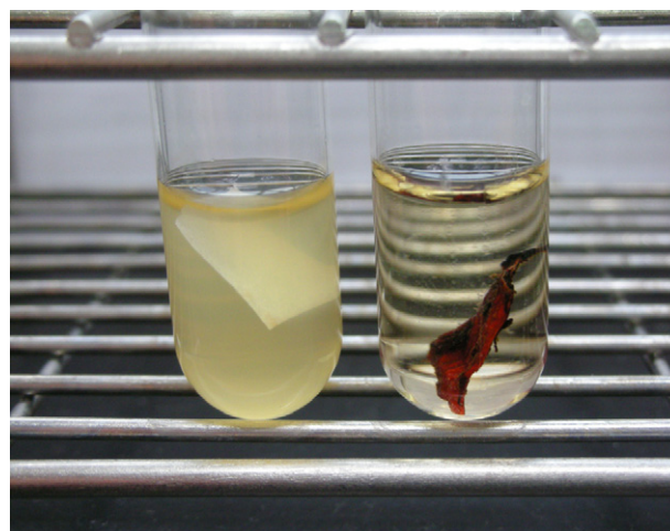
Fig. 4. Antibacterial activity of nonwoven PP fabric samples. Left: untreated nonwoven sample; right: bostrycin-treated nonwoven sample. Comparison with the untreated nonwoven sample, a clear bacteria-free solution was observed in bostrycin-treated nonwoven sample, indicating the bostrycin inhibited the growth of bacteria.
