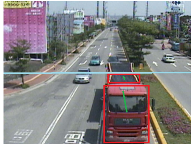
Fig. 15. Large trunk induces false-alarm detection.
