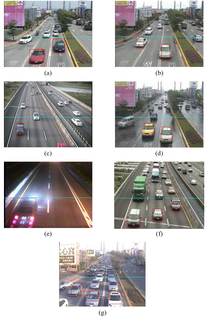
Fig. 14. Testing scenarios in various conditions. (a) Sunny day. (b) Cloudy day. (c) Shadow effects. (d) Rainy day. (e) Nighttime. (f) Heavy traffic on a highway. (g) Traffic jams in urban setting.
