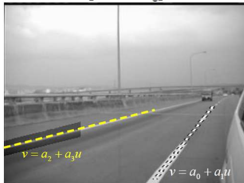
Fig. 14. Adaptive ROI of the far lane marking
