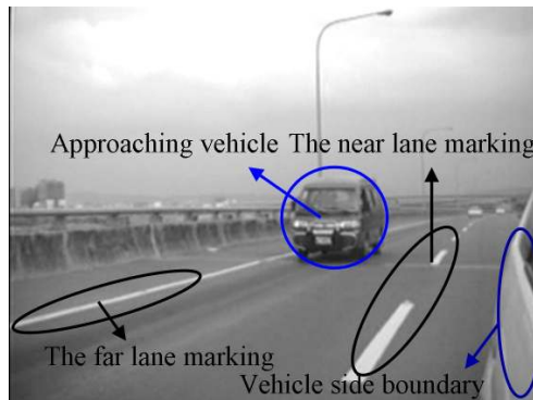
Fig. 11. The near lane marking and the far lane marking
