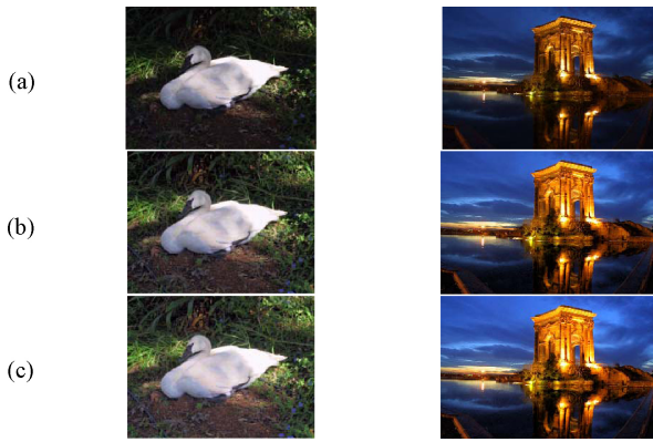
Fig. 14. Simulation results for S-BSPICE with early-stopping strategy. (a) Original image, and processing images (b) with early-stopping (left image: three iterations, right image: three iterations), (c) after the stopping criterion is satisfied (left image: 101 iterations, right image: 13 iterations).
