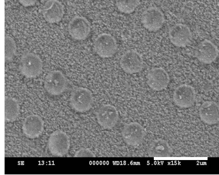
Fig. 2. SEM image of ITO etching at femtosecond laser power of 2 mW moving speed of 130 mm/s.
