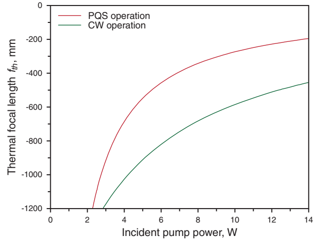
Figure 4 (online color at www.lasphys.com ) Numerical calculations of the thermal focal length versus the incident pump power for the CW and PQS cases
