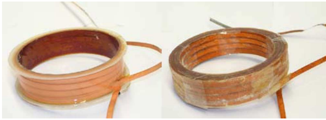
Fig. 4. (a) 88-turn coil without insulation. (b) 88-turn coil with 0.05-mm Kapton insulation (50% overlap).
