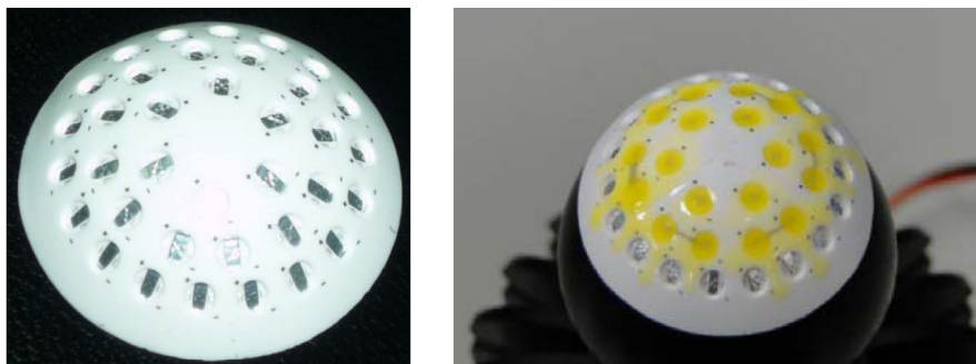
Fig. 10 Fabricated (a) curved ceramic substrate and (b) phosphor-coated LED.
