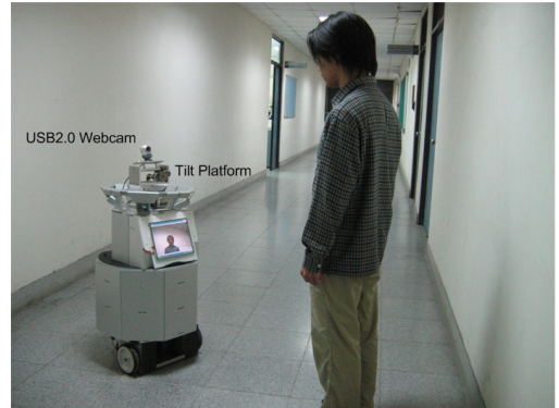
Fig. 3 The experimental mobile robot interacting with a user through face tracking.
