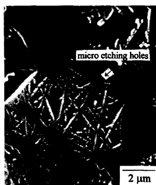
Fig. 2. Surface morphology of the AlN substrate before plating.
