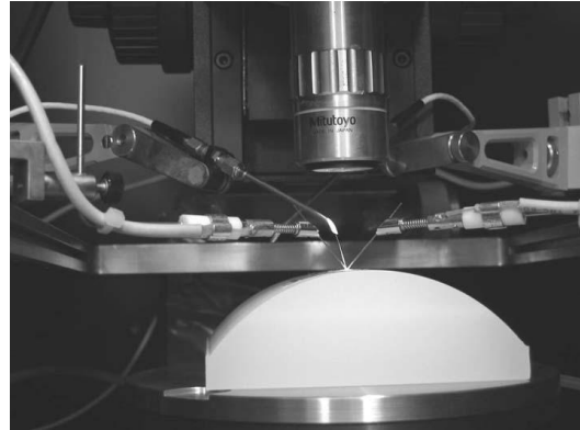
Fig. 11 Testing base and probes for bending measurement
