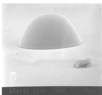
Fig. 12 Reflow microlens with diameter of 90 μm.
