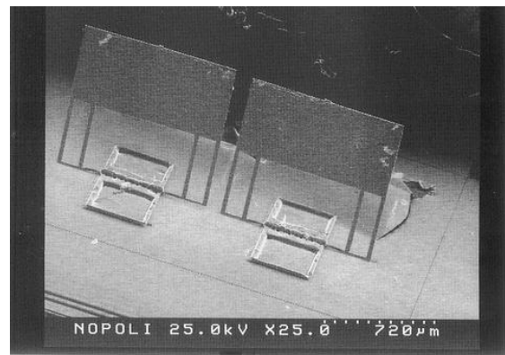
Figure 14: Lifted microstructures with hinge mechanism.
