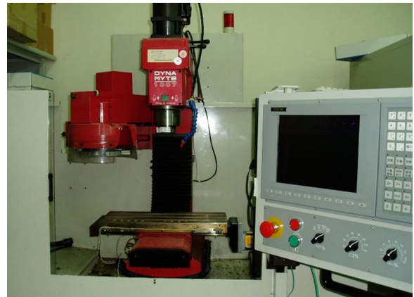
Fig. 10. DYNA DM1007 CNC machine tool.
