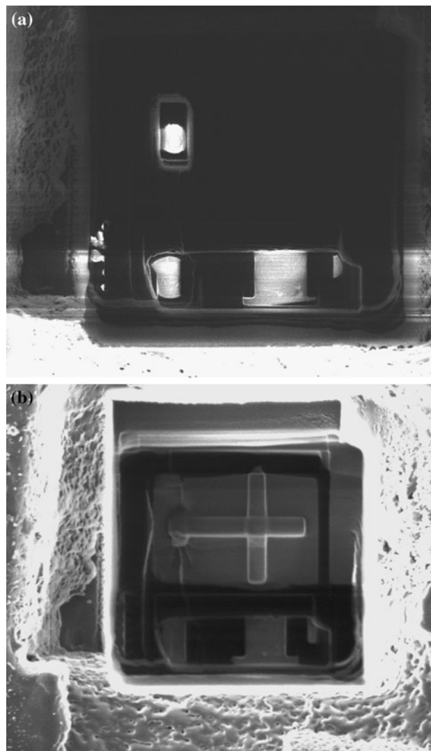
Fig. 6 a FIB micrograph of target IC metal exposure. b FIB micrograph of creation of probe pad on target IC metal
