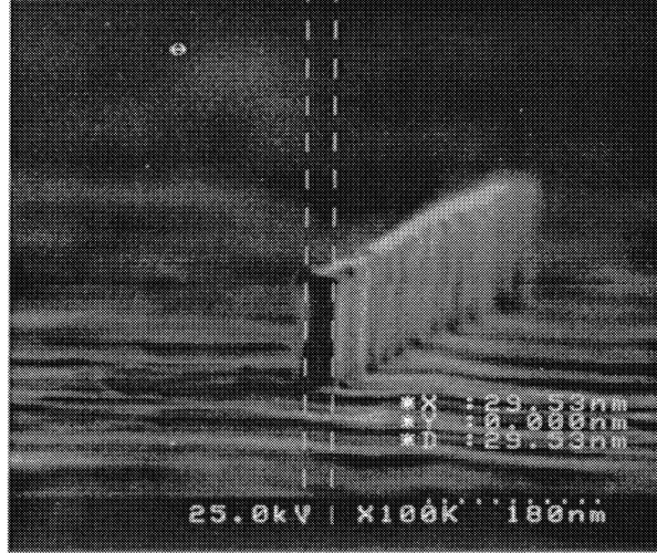
Figure 4 The sidewall SEM picture, gridline etching at 50°C.
