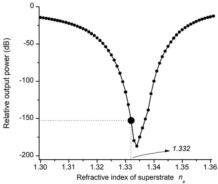
Figure 8. Relative output power versus superstrate index for an optimized Au-coated ARROW-B SPR sensor.
