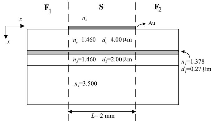
**Figure 2.** Basic structure of an ARROW-B SPR sensor.
