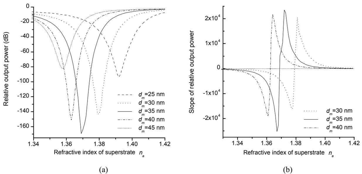
**Figure 4.** Dependence of the (a) relative output power and (b) the slope of that on the superstrate index.
