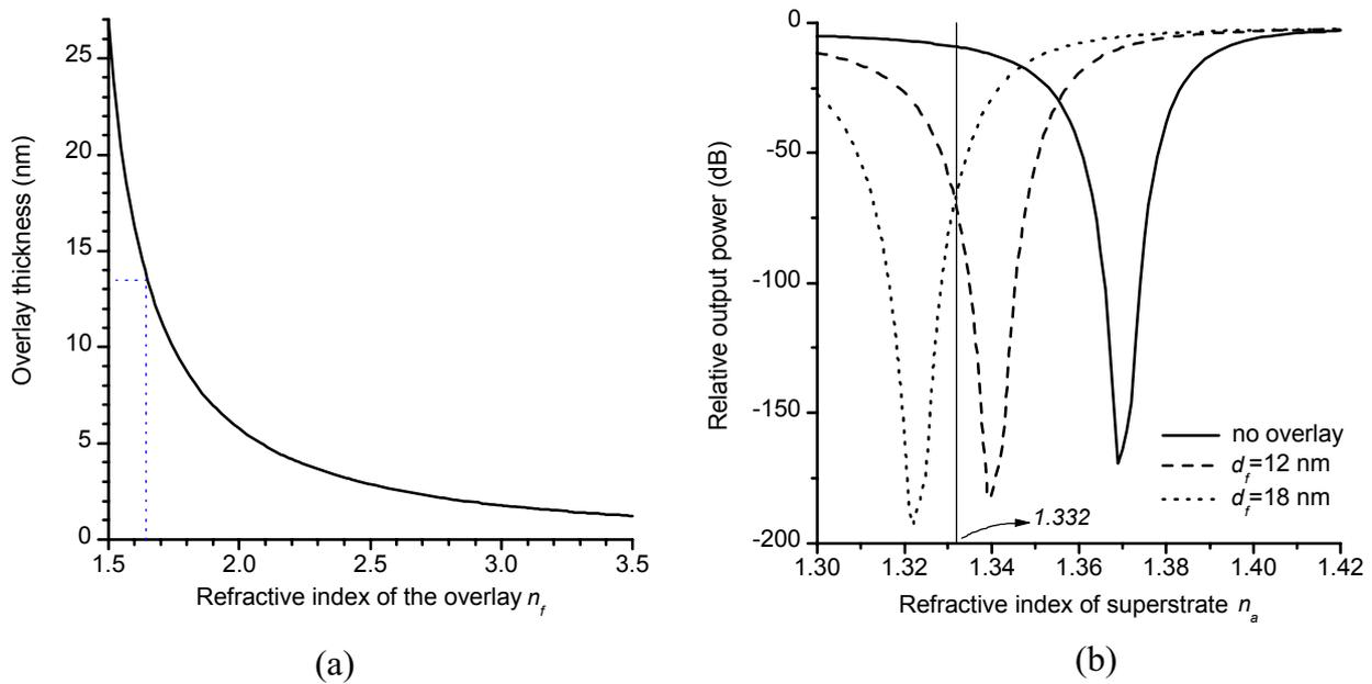
**Figure 6.** (a) Overlay thickness versus the refractive index of the overlay for  $n_{spr}=1.332$ . (b) Dependence of the relative output power on the superstrate index.
