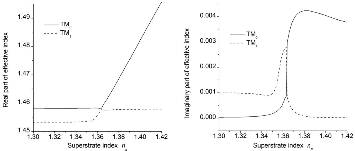
**Figure 3.** Real and imaginary parts of effective indices of the  $TM_0$  and  $TM_1$  in the sensing section of the ARROW-B SPR sensor.
