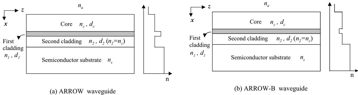
**Figure 1.** Structures and index profiles of ARROW and ARROW-B.
