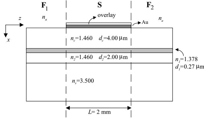
**Figure 5.** An Au-coated ARROW-B SPR sensor with an overlay.
