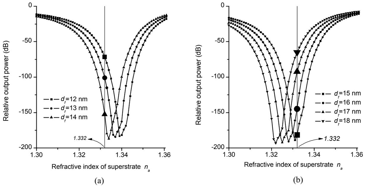
Figure 7. Relative output power versus superstrate index for various overlay thicknesses.
