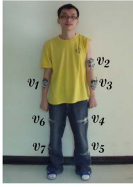
Fig. 2. An example of placing sensor nodes on a human body.
