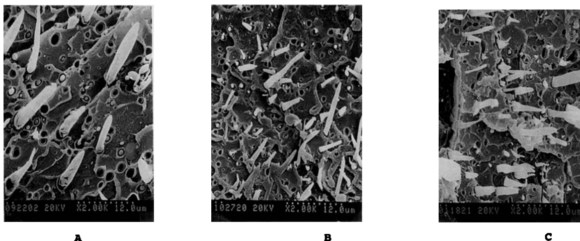
Figure 13 SEM morphologies of the fractured surfaces of the noncompatibilized and compatibilized Noryl/LCP = 85/15 blends. (A) Noryl/LCP = 85/15. (B) Noryl/LCP/SG5 = 85/15/5. (C) Noryl/LCP/SG5/Cat = 85/15/5/0.02.
