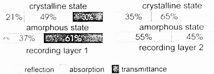
Fig. 2 Reflection, absorption and transmittance of layer 1 and 2 of a dual-layer optical disk
