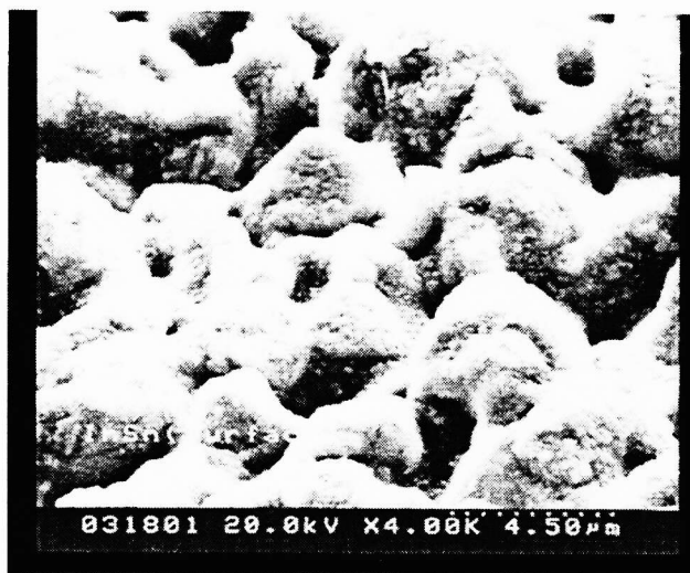
Fig.6 SEM photo of the surface morphology of as-deposited InSn solder film.
