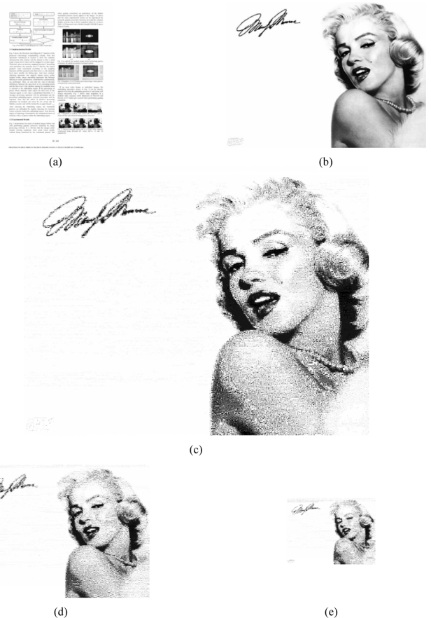
Fig. 9. Experimental result of grayscale mosaic image creation. (a) Secret image. (b) Target image. (c) Mosaic image created from a 1024 \times 768 secret image of (a) with RMSE = 30.86 . (d) Mosaic image created from a 768 \times 576 secret image of (a) with RMSE = 31.04 . (e) Mosaic image created from a 576 \times 432 secret image of (a) with RMSE = 30.7 .
