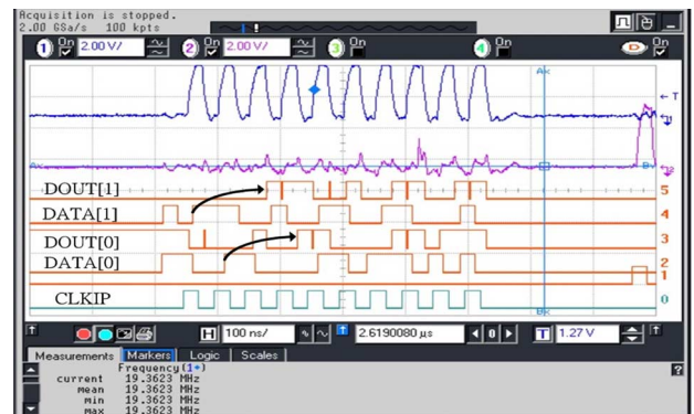
Fig. 19. Measurement results of state transition in the PIXEL_DATA state.
