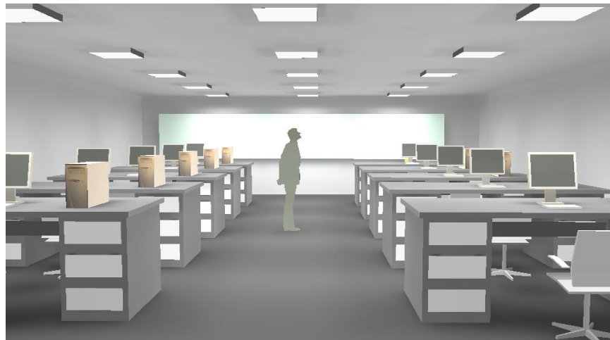
Fig. 17. Grayscale performance of the free-form flat panel lights in a computer classroom space.
