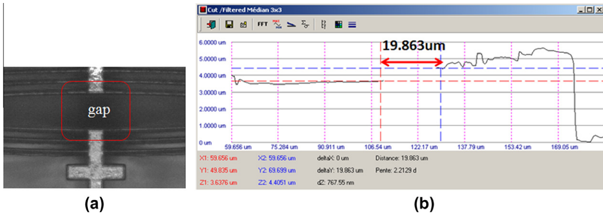
Fig. 15. (a) One side of the switch. (b) Measurement result by optical profiler.
