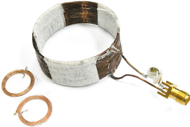
Fig. 3. Fabricated receiving and external coils.
