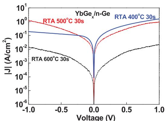
FIG. 2.  $J$ - $V$  characteristics of YbGe<sub>x</sub> contact on n-Ge wafer at different RTA temperatures. The ohmic behavior is useful for Ge nMOS.
