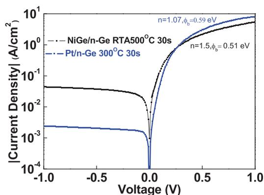
FIG. 1.  $J$ - $V$  characteristics of NiGe and Pt contact on n-Ge wafer. The Schottky diode characteristics are suitable for Ge pMOS, but not for Ge nMOS.
