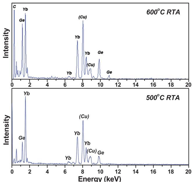
FIG. 4. EDS profile for YbGe<sub>x</sub>/n-Ge contacts formed at 500 °C and 600 °C RTA.
