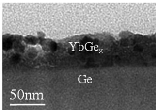
FIG. 3. Cross-sectional TEM image of YbGe<sub>x</sub> on n-Ge wafer after 600 °C RTA, with smooth interface and without contact metal spiking.
