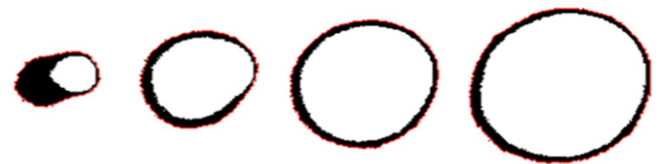
Fig. 5. Result of edge detection of each dark fringe.
