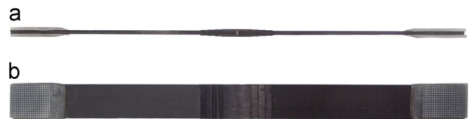
Fig. 3. Photos of stepwise patch joint (SDLJ-2): (a) side view and (b) top view.
