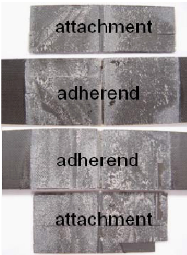
Fig. 7. Failure surfaces of SDLJ-2 sample.
