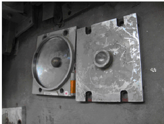
Fig. 5. (a) Test model of single-storey with FPS isolation system and (b) friction pendulum system used in the test.
