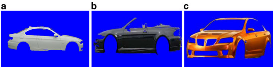
Fig. 4 a–c The extracted car body candidates of the a white, b black, and c orange cars after the process of the SARM algorithm
