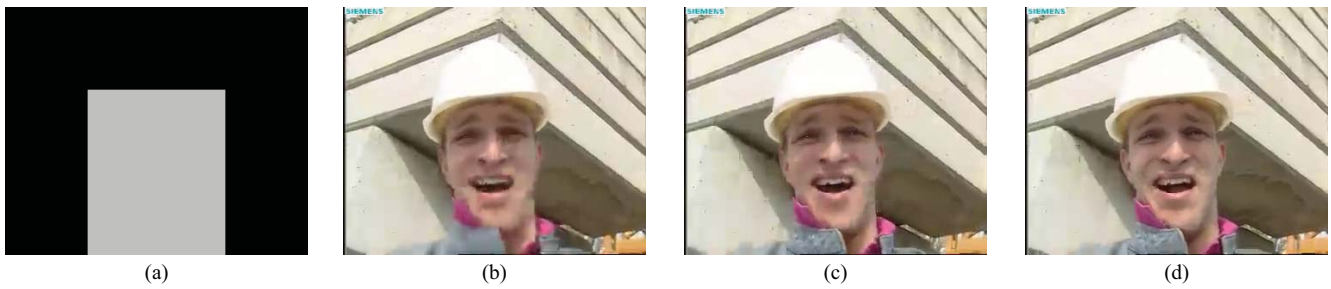
Fig. 1. Basic concept of the quality-regulable coding system. The quality of ROI regions can be adjusted based on user's target quality under the constraint of the same bitrate. (a) ROI (white region) and non-ROI (black region). (b) ROI quality:50 and non-ROI quality:70 Bitrate:100. (c) ROI quality:60 and non-ROI quality:60 Bitrate:100. (d) ROI quality:70 and non-ROI quality:50 Bitrate:100.
