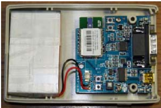
Figure 8 WSN module – Jennic-HSCC (see online version for colours)
