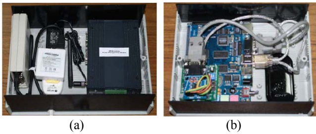
Figure 10 Wireless gateways: (a) WSN/Wi-Fi (b) WSN/3G (see online version for colours)
