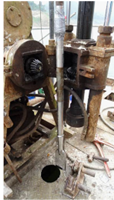
Fig. 10 The fully assembled \Delta DMT
