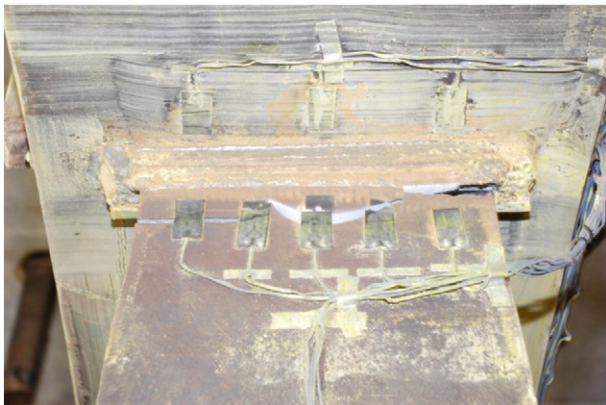
Fig. 5. Specimen UR beam top flange fracture (first test).
