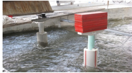
Figure 4. Single bridge column test.
