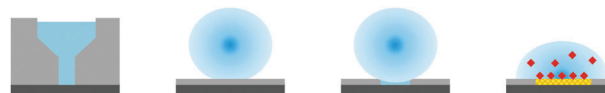
Fig. 7 Common embodiments of the on-target pre-concentration of samples before the analysis by MALDI-MS or LDI-MS. The samples can be loaded into microwells on the MALDI target, deposited onto a hydrophobic target, deposited into hydrophilic sites surrounded by the hydrophobic area, or incubated with a molecular recognition surface on the MALDI target.
