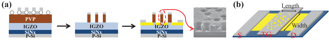
Fig. 1. (a) Fabrication process of the DG-NDD a-IGZO TFT and the SEM image in porous structure. (b) 45° view of the device structure. Channel width and length are defined by the patterned of the IGZO and the TG metal.
