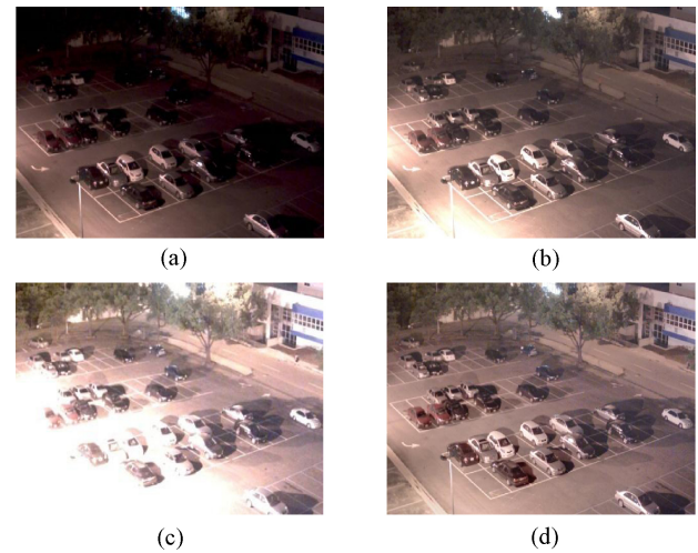
Fig. 3. (a) Image with a short exposure. (b) Image with a medium exposure. (c) Image with a long exposure. (d) Fusion result of the images in (a), (b), and (c).
