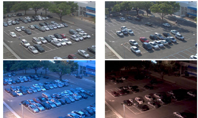
Fig. 1. Challenges for robust vacant parking space detection, including perspective distortion, inter-object occlusion, shadow effect, variations of lighting condition, and insufficient illumination at night.
