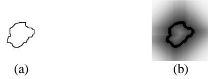
Fig.7. (a) A boundary of an extracted region (b) The distance map of (a). The brighter points mean the longer distance from the contour. The points inside the contour are set to negative distance.
