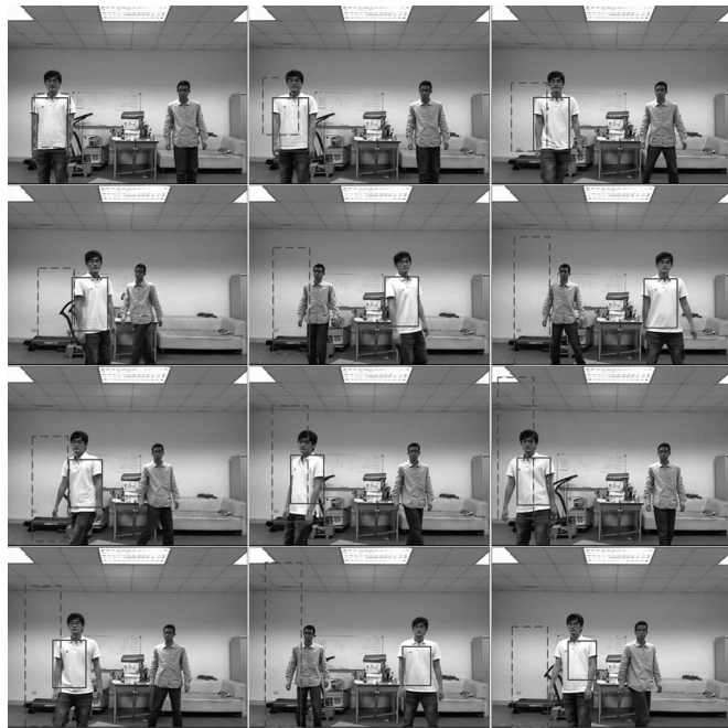
Fig. 13. Results of the body tracking using meanshift algorithm (dashed line) and the proposed method (solid line), where frames 1, 10, 40, 60, 100, 130, 185, 198, 220, 240, 336, and 398 are listed.
