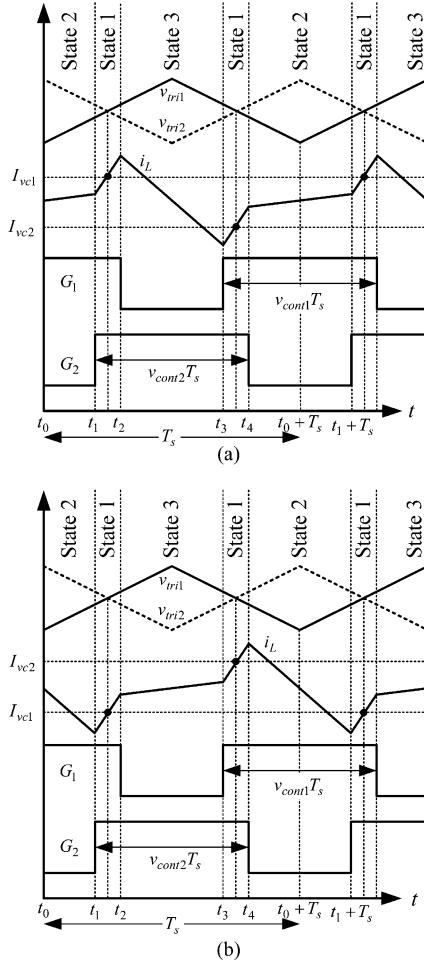
Fig. 6. The illustrated waveforms for the case of  $v_{cont1} + v_{cont2} > 1$ : (a) when  $v_{C1} > v_{PV} > v_{C2}$ ; (b) when  $v_{C2} > v_{PV} > v_{C1}$ .
