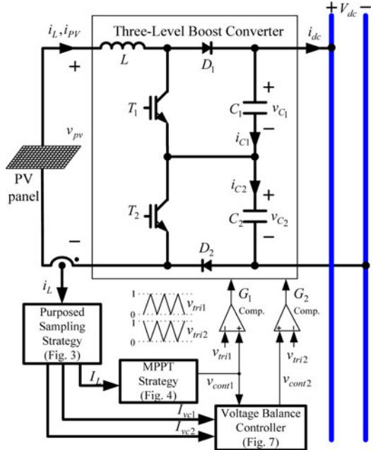
Fig. 1. PV-fed three-level boost-type converter with the proposed voltage balancing control.
