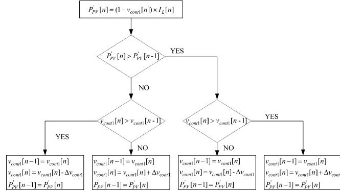
Fig. 4. Proposed MPPT algorithm with only sensing inductor current.
