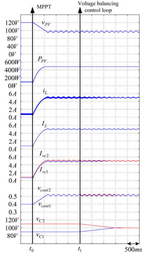
Fig. 8. Simulated results for the proposed MPPT and voltage balancing control methods.
