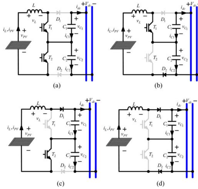
Fig. 2. Possible switching states in three-level boost-type converter: (a) state 1; (b) state 2; (c) state 3; and (d) state 4.
