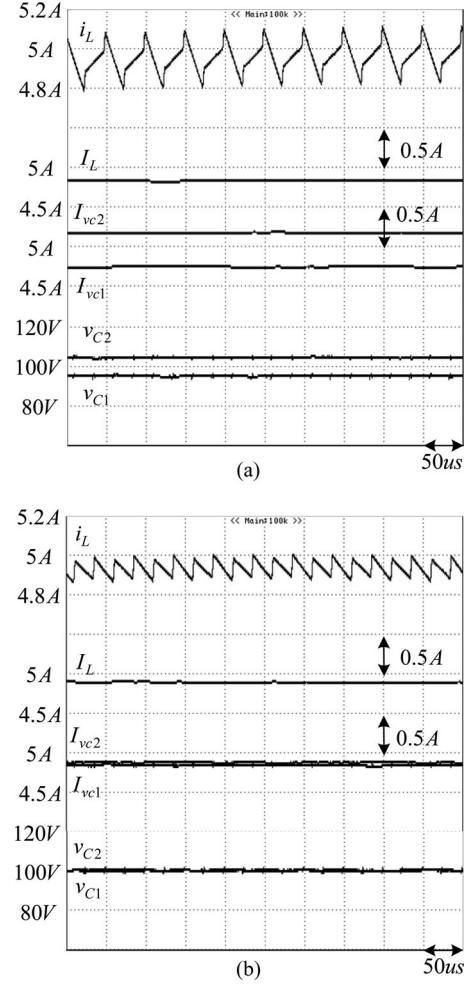
Fig. 10. Enlarged steady-state waveforms (a) before the voltage balancing control loop is applied and (b) after the voltage balancing control loop is applied.
