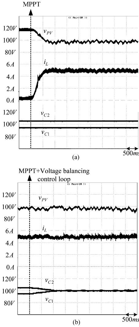
Fig. 9. Experimental results (a) with the proposed MPPT control and (b) with the proposed MPPT and voltage balancing control loop.
