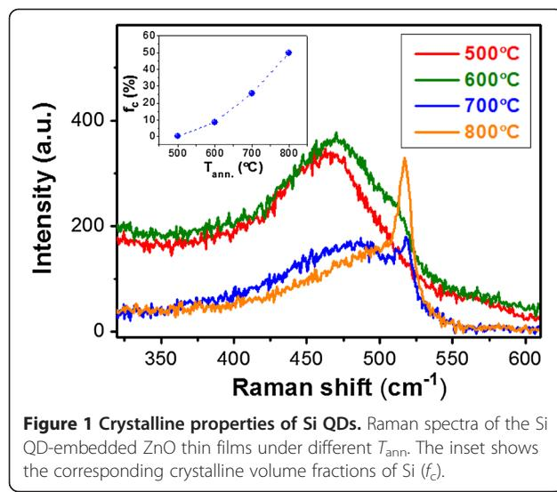
**Figure 1** Crystalline properties of Si QDs. Raman spectra of the Si QD-embedded ZnO thin films under different  $T_{\text{ann}}$ . The inset shows the corresponding crystalline volume fractions of Si ( $f_c$ ).
