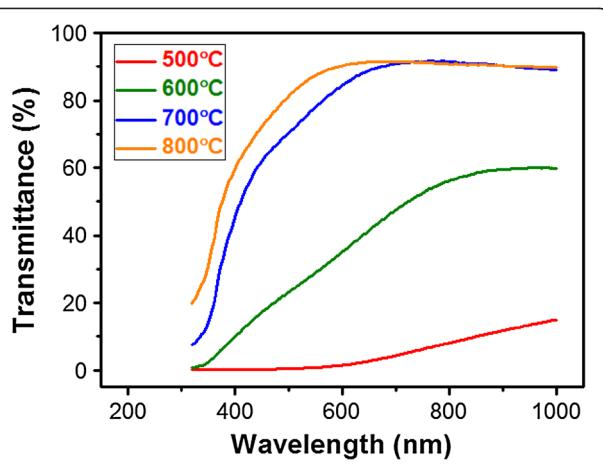
**Figure 3 Optical properties.** Optical transmittance spectra of the Si QD-embedded ZnO thin films under different  $T_{\text{ann}}$ .
