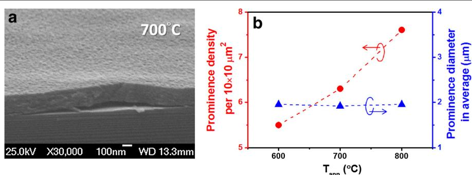
**Figure 4 Thin film image.** (a) Cross-sectional SEM image and (b) local film prominence density and diameter in average for the Si QD-embedded ZnO thin films after annealing.
