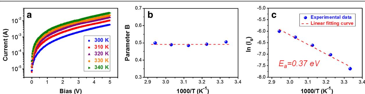
**Figure 6 Carrier transport mechanism.** (a) Forward  $I$ - $V$  curves for different measurement temperatures, (b) the parameter  $B$ , and (c) Arrhenius plot of  $\ln(I_s)$  versus  $1/1000/T$  for the Si QD-embedded ZnO thin film annealed at 700°C.
