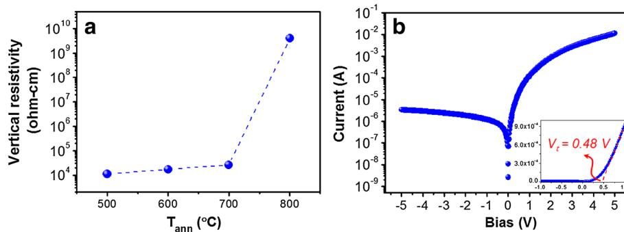
**Figure 5 Electrical properties.** (a) Vertical resistivity of the Si QD-embedded ZnO thin films under different  $T_{\text{anno}}$ . (b) Logarithmic  $I$ - $V$  curve of the sample annealed at 700°C. The inset shows the linear  $I$ - $V$  curve in magnification.
