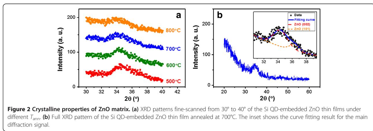
**Figure 2** Crystalline properties of ZnO matrix. (a) XRD patterns fine-scanned from 30° to 40° of the Si QD-embedded ZnO thin films under different  $T_{\text{ann}}$ . (b) Full XRD pattern of the Si QD-embedded ZnO thin film annealed at 700°C. The inset shows the curve fitting result for the main diffraction signal.
